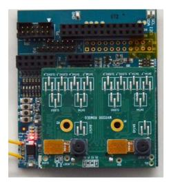
The Peephole device equipped with a AMX 208 module (Sony).
