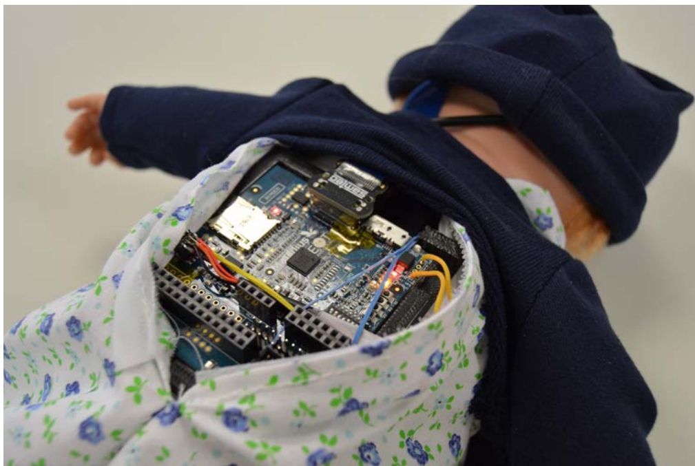
Figure 4: Back side of the Doll with EoT Board
