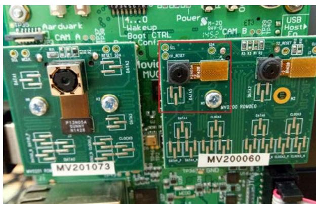
Figure 6-17: MIPI IMX208 camera used for EoT DevBoard.
