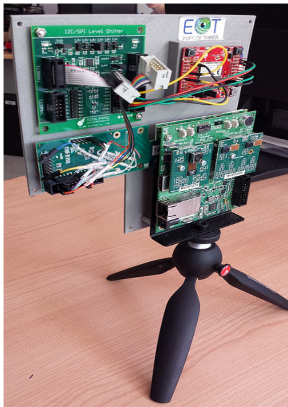
Figure 5: Wi-Fi HW rig on MV0182.
