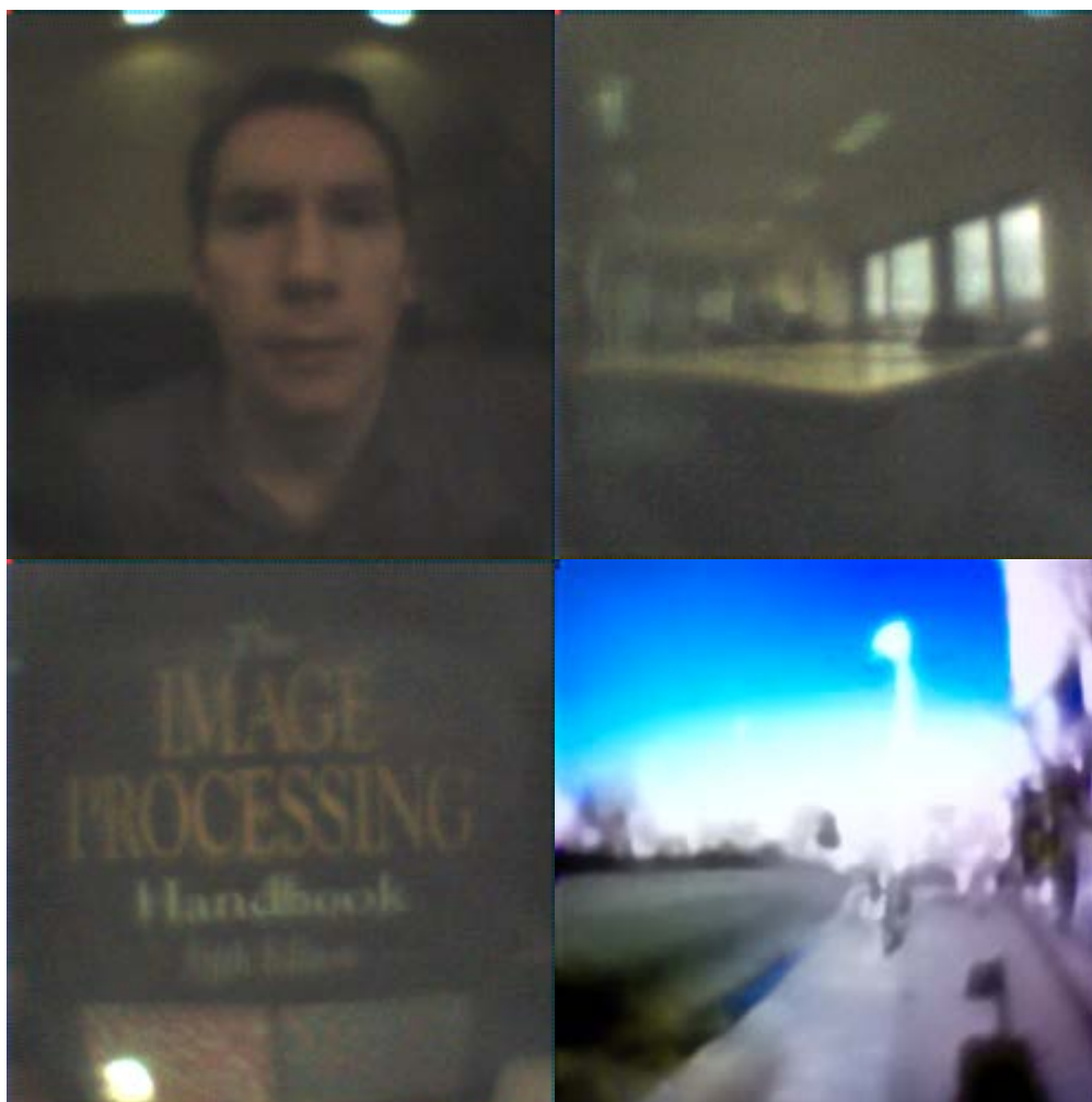
Figure 5.11: Sample debayered images from NanEye sensor (after basic image processing)
